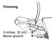
SCALPING - The scalping technique re-moves unwanted vegetationdown to the ground. Hold the bottom of the trimmer head about 3 in. (8 cm) above the ground and at an angle. Allow the tip of the line to strike the ground around trees, posts, monuments, etc. This technique increases line wear.
